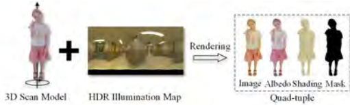
Fig. 4 For each pair of the illumination map and 3D scan model, a quad-tuple (i.e., image, shading, albedo, and mask) is rendered.
