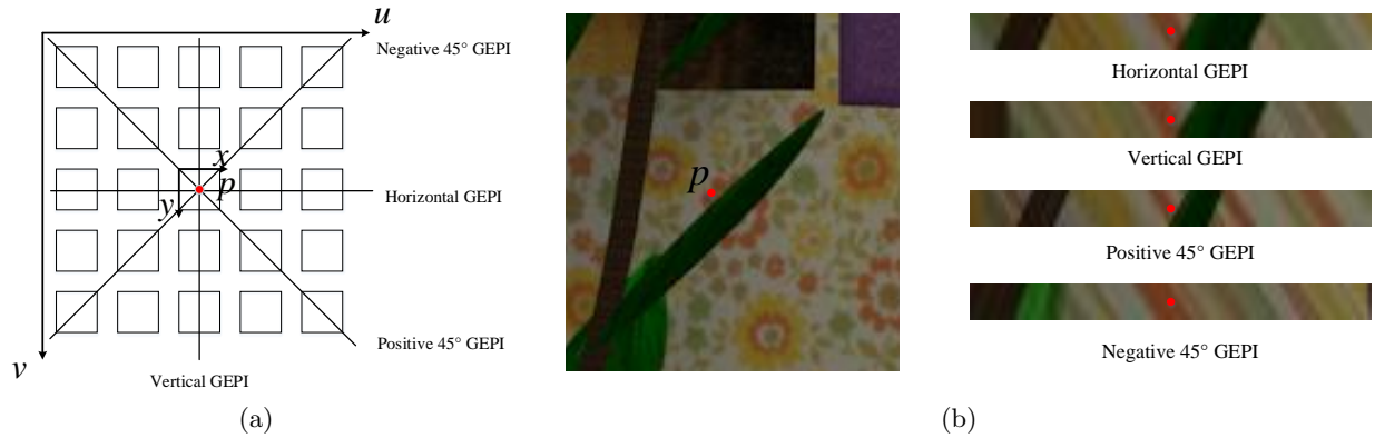
Figure 2. The GEPI representations in light field. (a) shows how GEPIs are obtained in different directions. (b) shows 4 GEPIs in four directions. It is noticed there is no occlusion in -45^\circ GEPI, as the occlusion boundary near p has the same orientation as GEPI direction.
